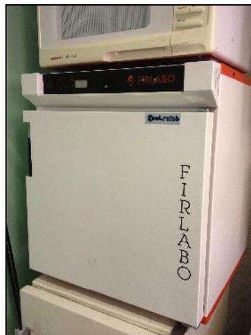
Figure 18 : Etuve (Controlab Firlabo)
